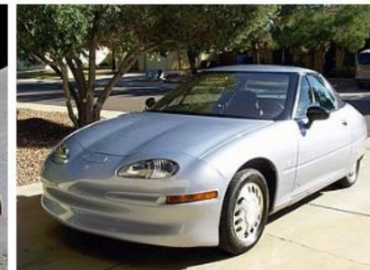
The General Motors EV1 , one of the cars introduced due to a California Air Resources Board (CARB) mandate, had a range of 260 km (160 miles) with NiMH batteries in 1999.
