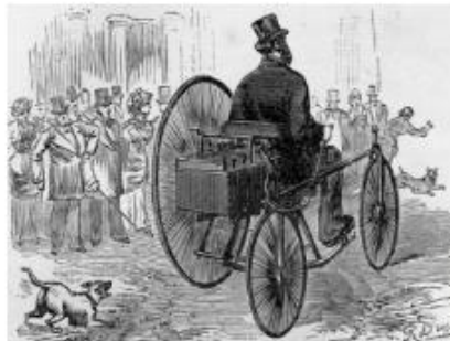
Gustave Trouvé's personal electric vehicle (1881), the world's first publicly presented full-scale electric car powered by an improved Siemens motor
