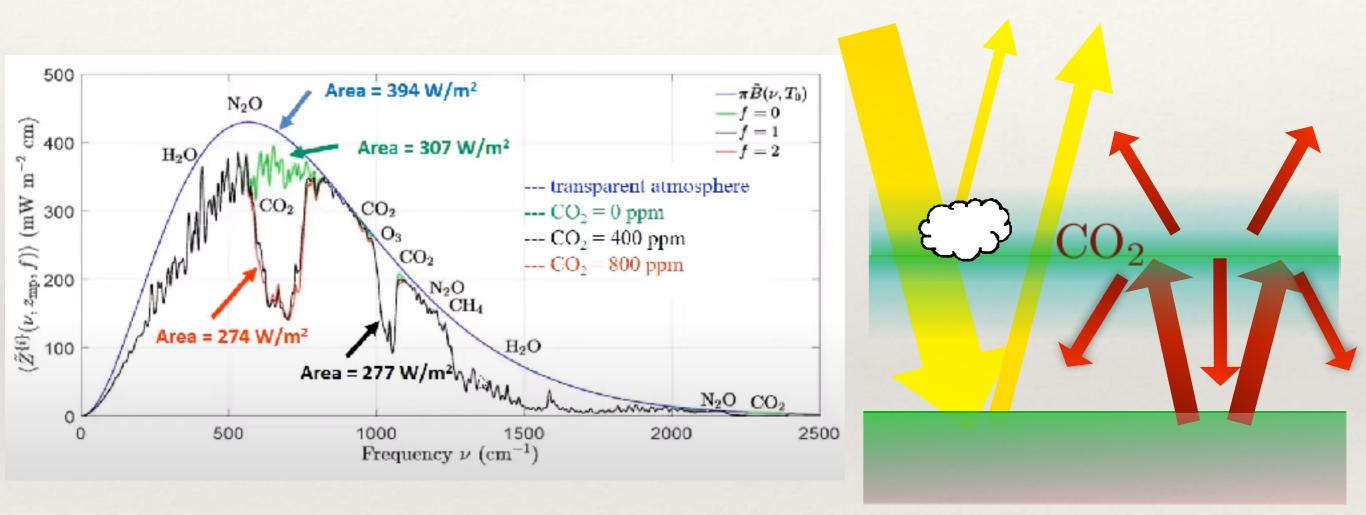
\* To compensate for the reduced radiation to space, the surface temperature has to increase. If everything stays the same,  $\Delta T = 1.0-1.2^{\circ}C$  per CO<sub>2</sub> doubling.
