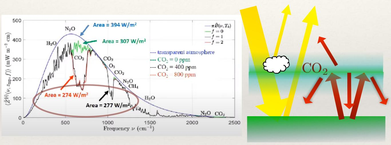
Adding more greenhouse gases reduces radiation going to space by 3-4 W/m<sup>2</sup> (compared with 240 W/m<sup>2</sup> that reaches the surface)
