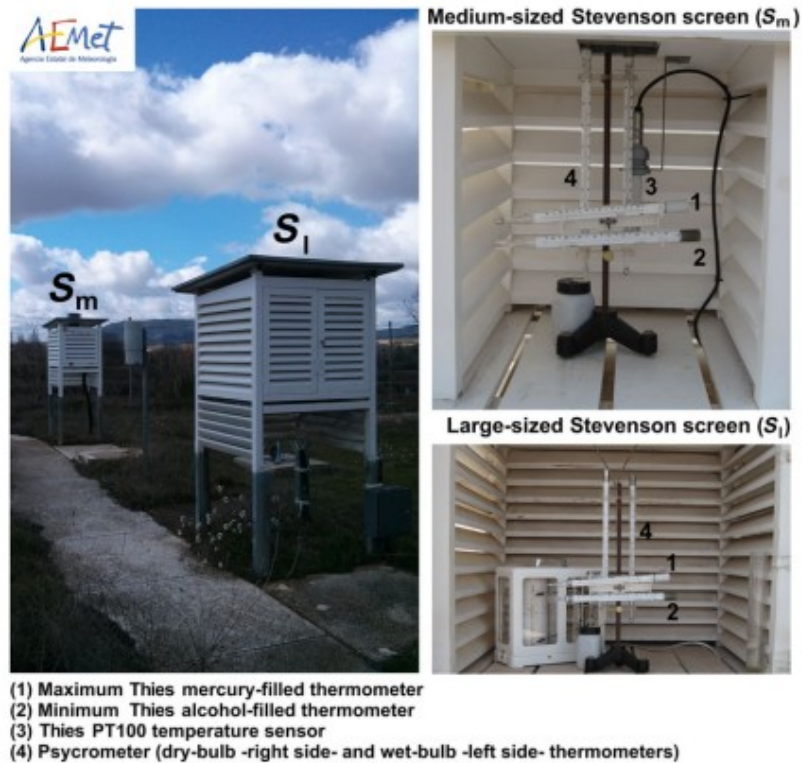
Figure 2. The medium- and large-sized Stevenson screens with the corresponding set of thermometers used in the field intercomparison at the Calamocha first-order meteorological station.
