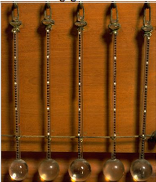
Abb. 3a: Thermometer (17.Jhdt) und modernes Infrarot-Thermometer Links: Ferdinand II de' Medici [attr.] Museo Galileo , Termometri cinquantigradi inv 85 IF 46774 , CC BY-SA 4.0 Rechts: Hedwig Storch , 1024 Pyrometer-8445 , CC BY-SA 3.0
