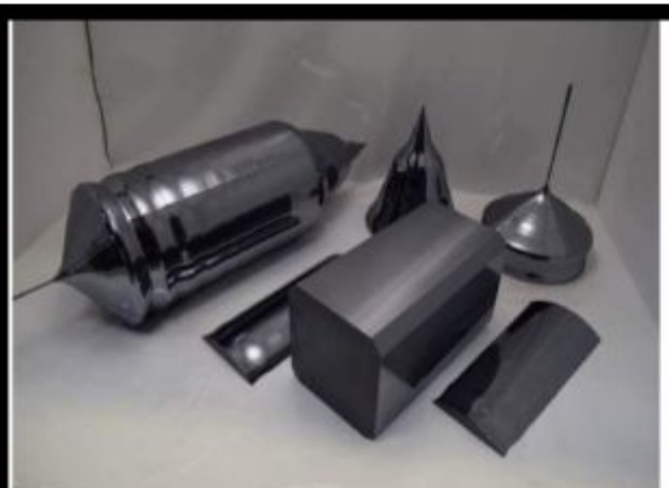
Czochralski process whole ingot (left), and brick and chords after sawing (right), crown and tail (upper right) ( SVM )
