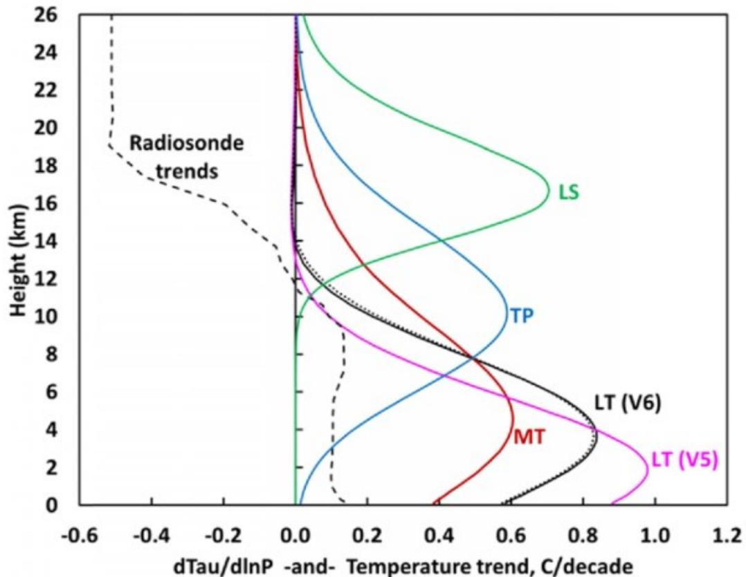
**Fig. 2.** MSU weighting functions computed from radiative transfer theory for the chosen reference Earth incidence angles, and the resulting LT averaging kernels computed from a linear combination of the MT, TP, and LS weighting functions (the dotted line is for LT computed from AMSU). Also shown is an estimate of the global temperature trend profile (dashed) from the average of RAOB-CORE and RATPAC radiosonde data used to determine the stratospheric sensitivity of the new LT averaging kernel.
