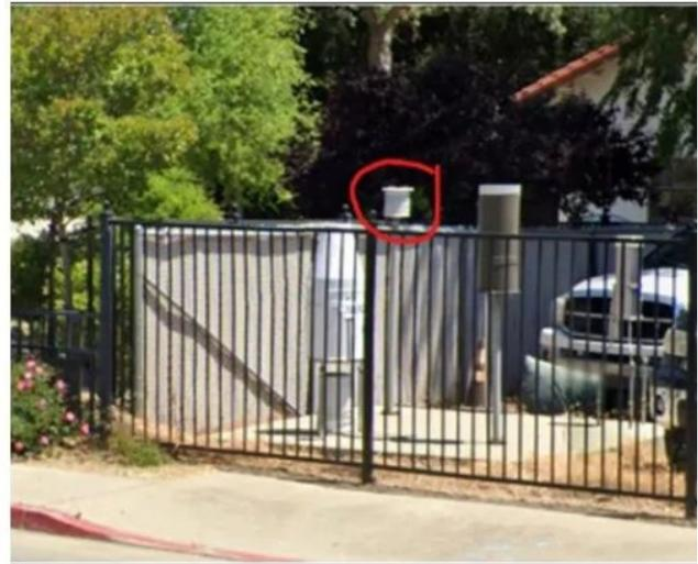
**“The sensor should be at least 100 feet from any paved or concrete surface.”**
