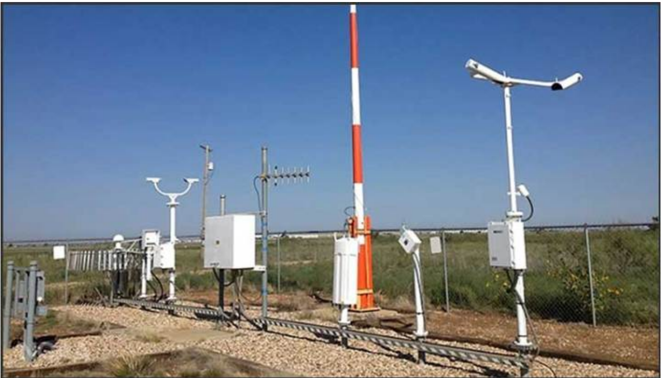
A NOAA Automated Surface Observing System (ASOS) weather station at the Childress Municipal Airport in Childress, Texas. ASOS stations constantly monitor weather conditions on Earth's surface. More than 900 stations across the United States report data about sky conditions, surface visibility, precipitation, temperature and wind up to 12 times an hour. Credit: NOAA
