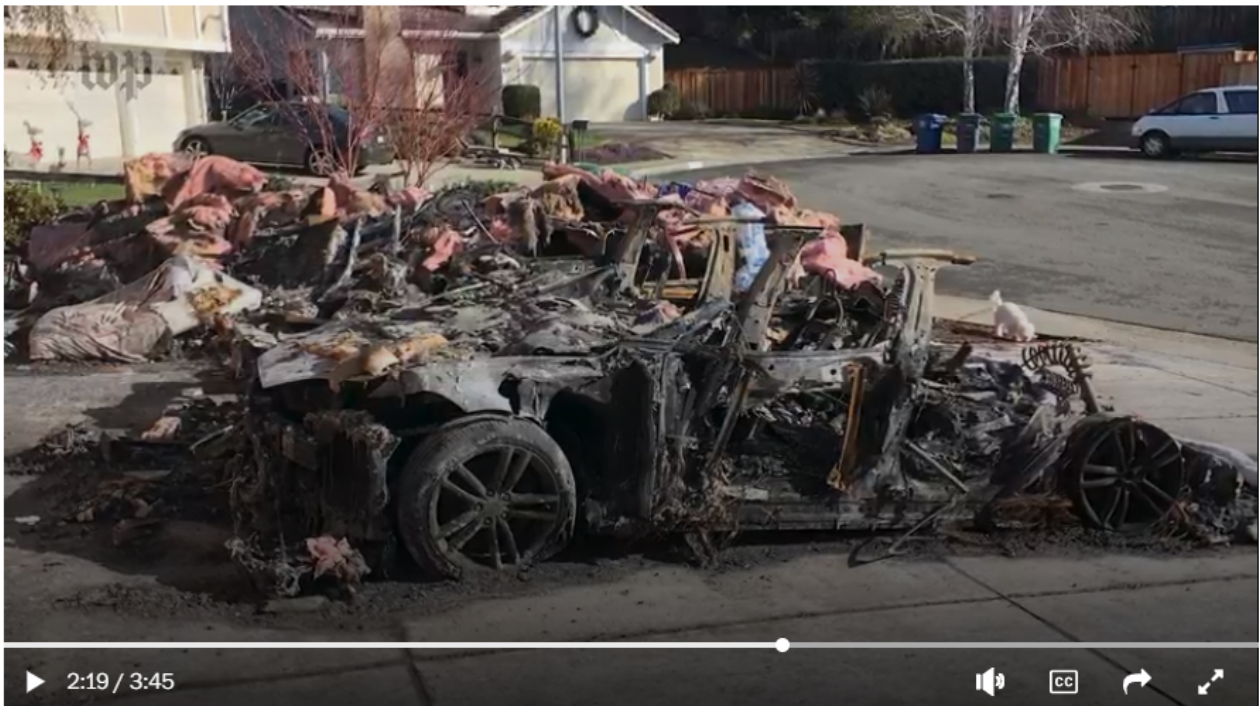
A fire inspection report cited the Tesla Model S's thermal management system and a fault in the electrical system as two possible causes in the fire. (Jonathan Baran/The Washington Post)
