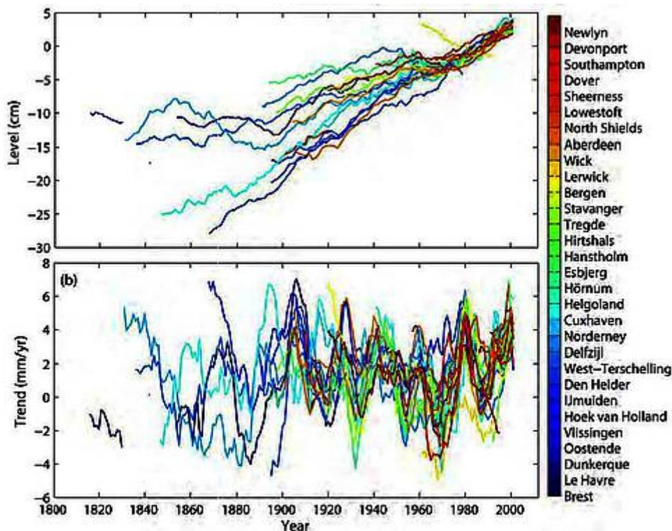
**Fig. 10.** (a) 20-year running means for all records, after correcting for GIA (for presenting purposes all records were adjusted to have zero mean for the 50-yr period from 1960 to 2009); (b) running 20-year linear trends for all records after correcting for GIA.
