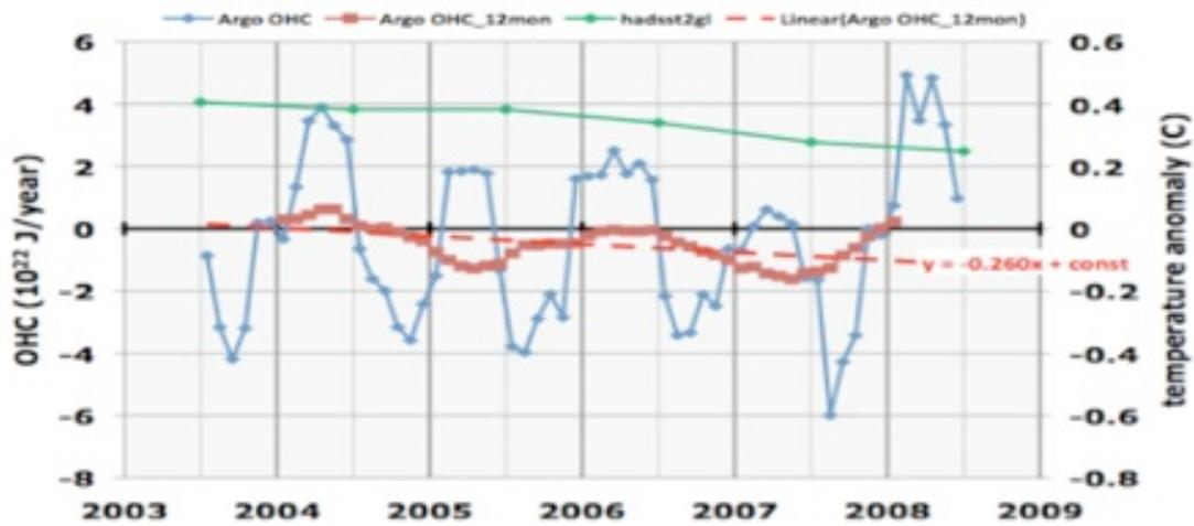
Figure 1. Ocean heat content from Argo (left scale: blue, original data; red, filtered) and ocean surface temperatures (right scale, green). Conversion of the OHC slope to  $W/m^2$  is made by multiplying by 0.62, yielding  $-0.161 W/m^2$ .
