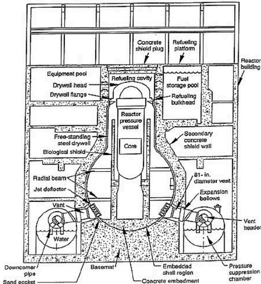
Figure 20. Mark I General Electric, GE BWR Containment.
